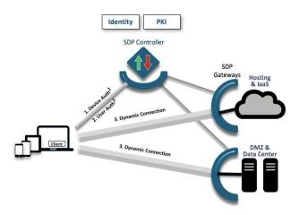
Fig. 5. Architecture for software defined perimeter (SDP).
